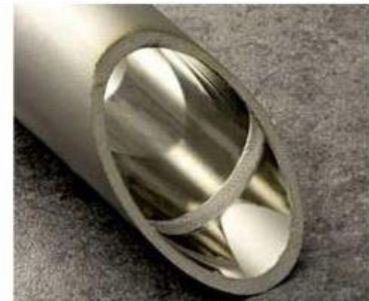
Cut away shows internal quality of orbital welding
